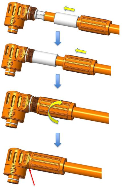
No gap between connector body and backshell
