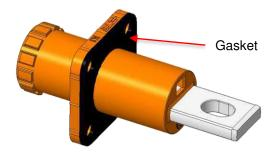
5.2. Tighten receptacle connector onto the panel with M4 screws (recommended torque as 0.8±0.1N.m)
